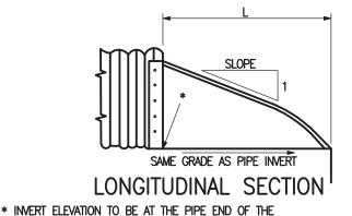
STANDARD END SECTION. ELEVATIONS TO BE NOTED ON CONSTRUCTION PLANS.
