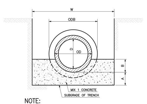
WHEN 2 TIER TRENCH SUPPORT IS REQUIRED, ADD 24" TO "W" FOR CALCULATING THE AMOUNT OF PAVING NEEDED FOR TRENCH REPAIR.
