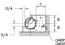
CARRY CONCRETE TO UNDISTURBED EARTH.
