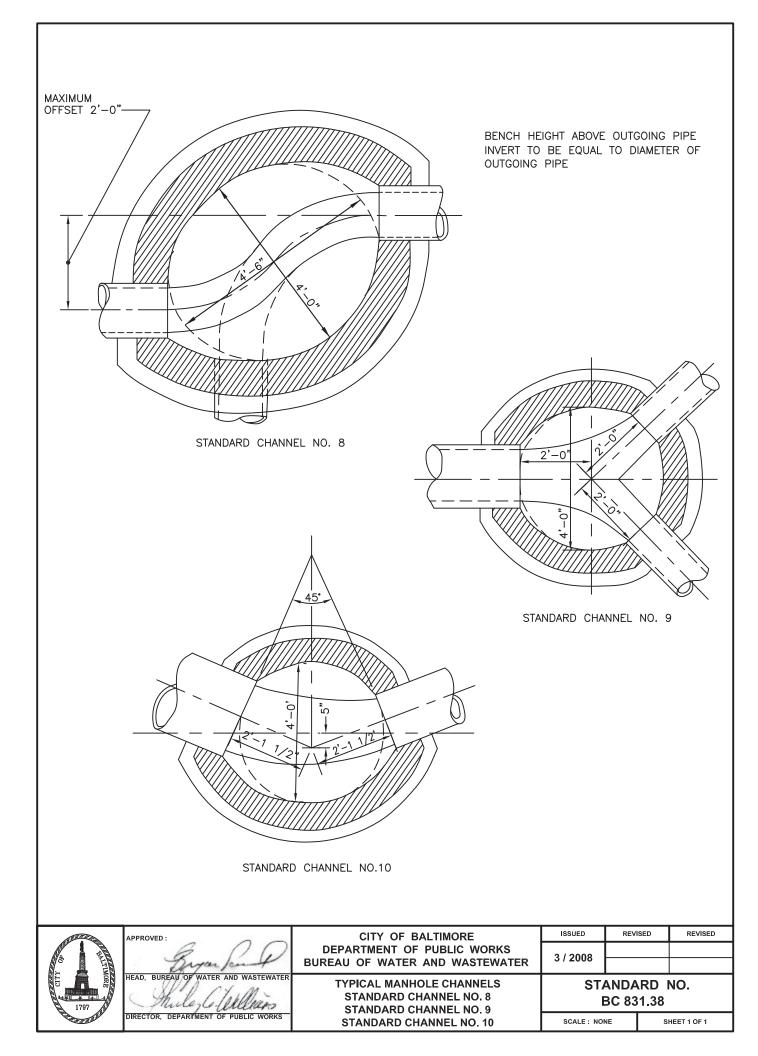
BENCH HEIGHT ABOVE OUTGOING PIPE INVERT TO BE EQUAL TO DIAMETER OF OUTGOING PIPE
